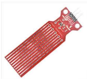
Figure 5: HW-038 Water Level Sensor
